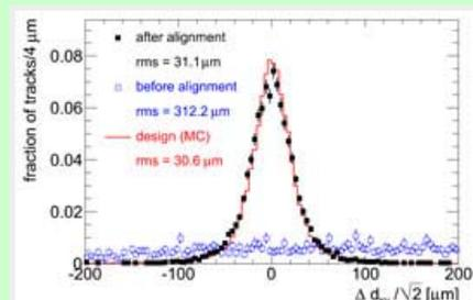
Impact parameter resolution of cosmic muon tracks passing near the nominal interaction region. Performance after alignment, before alignment, and design are compared
